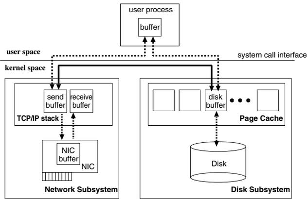
Fig. 1. The Architecture of I/O subsystem in Linux 2.4.
