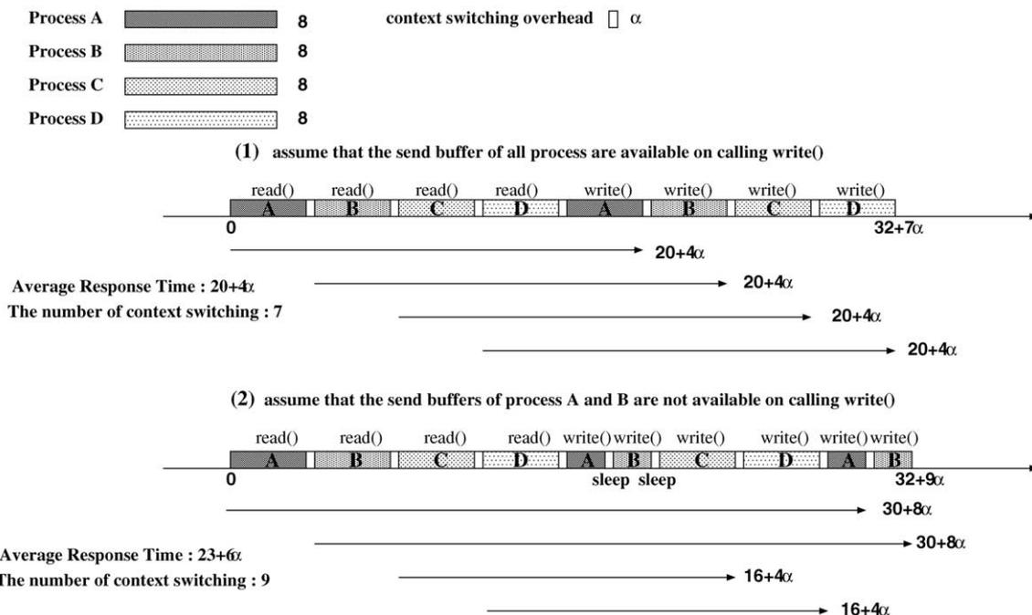
Fig. 3. Long response time during processing a request.
