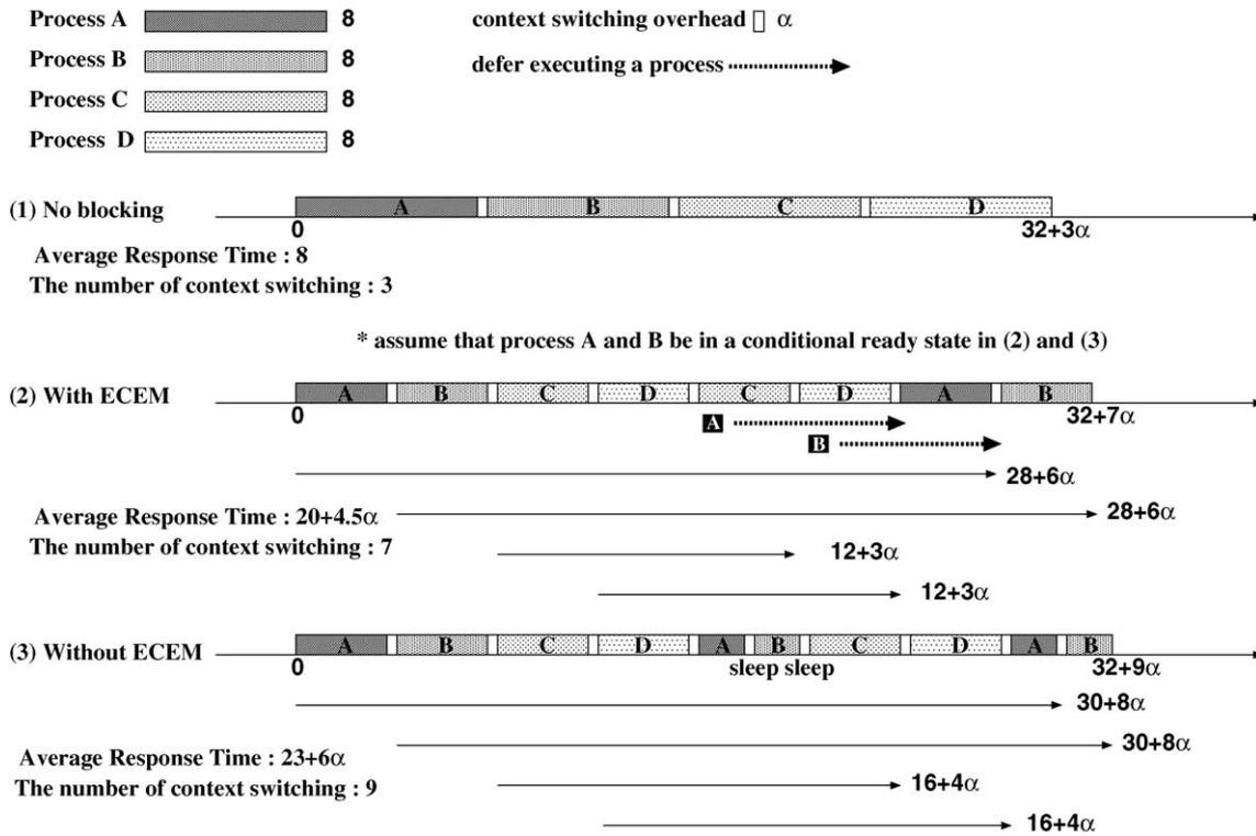
Fig. 7. Time diagram during request processing with ECEM.
