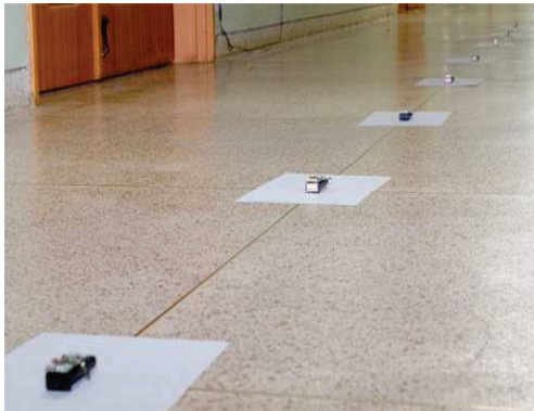
Figure 8: Topology used in experiments: 7-hop indoor network with one source and one sink. All nodes are 4m apart.
